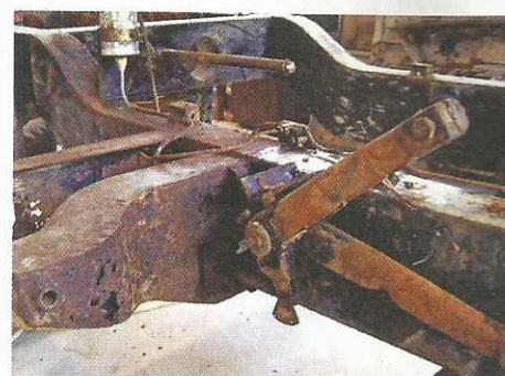
Chassis outriggers were all past saving, but the main body of the chassis had survived pretty well
