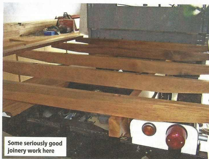
Chassis outriggers were all past saving, but the main body of the chassis had survived pretty well
